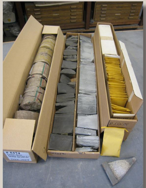
Figure 1. Left to Right: Whole core, slabbed core, and samples.
