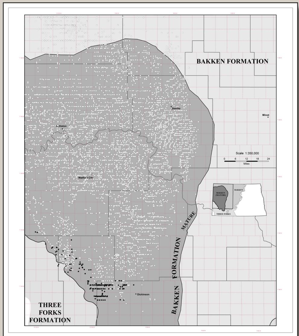
**Figure 3.** Horizontal oil wells (dots) that are producing or have produced from the Bakken Petroleum System. The Whiting's Pronghorn wells are in black. Other companies have followed Whiting's lead and drilled Pronghorn wells in the vicinity of Whiting's play.
